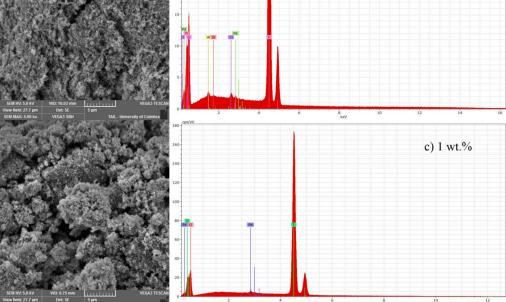
Figure 1. SEM-EDS analysis for catalysts (a) 0.1% Pd-TiO<sub>2</sub>; (b) 0.5% Pd-TiO<sub>2</sub>; and (c) 1% Pd-TiO<sub>2</sub>.
