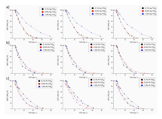
**Figure 2.** Normalized concentration of individual parabens MP, EP, PP as a function of TOD during photocatalytic ozonation for different noble metal loads of (**a**) Ag-TiO<sub>2</sub>; (**b**) Pd-TiO<sub>2</sub>; (**c**) Pt-TiO<sub>2</sub>.
