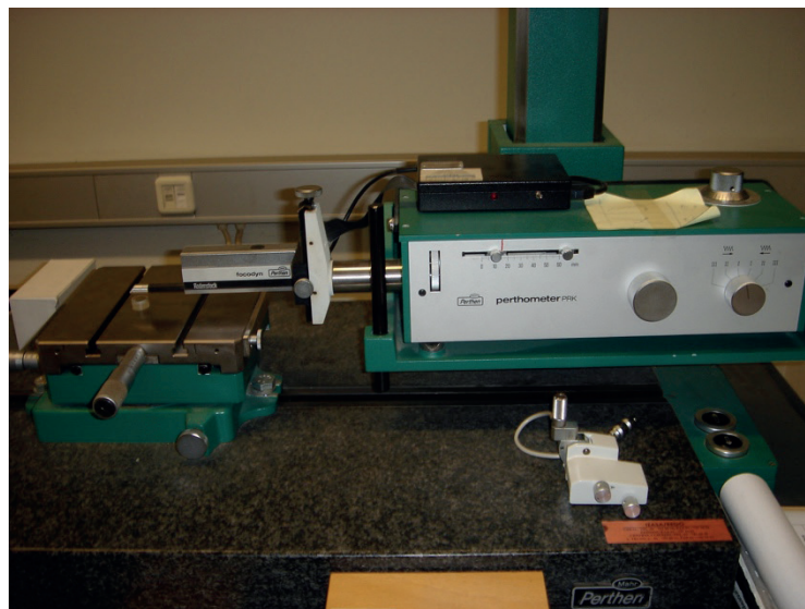
Figure III.3. Perthen S4P Rugosimeter 2D with mechanical probe and laser, Mahr, Germany. Hosted in Pedro Nunes Institute, Testing, Wear and Materials Laboratory (LED&MAT).
