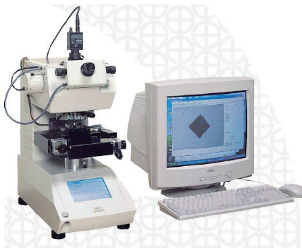
Figure III.1. Micro Vickers Tester HMV-2 Shimadzu, Japan. Hosted in Pedro Nunes Institute, Testing, Wear and Materials Laboratory (LED&MAT). Image reproduced from: https://www.shimadzu.com/ .
