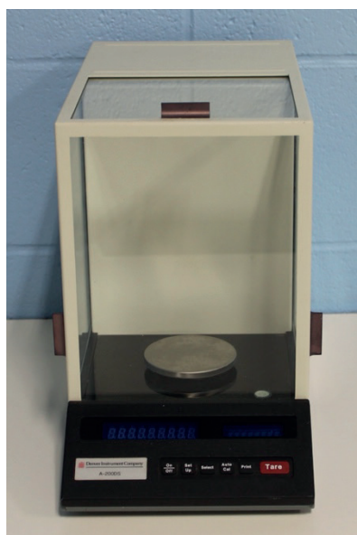
Figure III.2. Denver Instrument A-200DS Analytical Balance, USA. Hosted in Pedro Nunes Institute, Testing, Wear and Materials Laboratory (LED&MAT).
