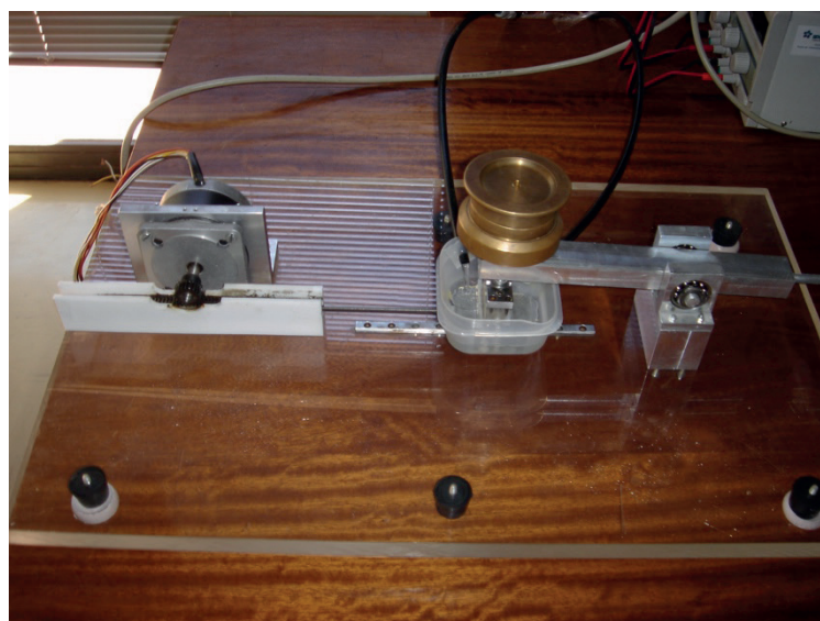
Figure III.4. Two-body alternative sliding equipment with parameterizable stroke, speed and applied load, designed by Pedro Nunes Institute, Testing, Wear and Materials Laboratory (LED&MAT).
