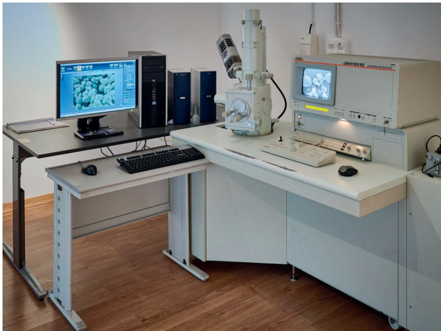
Figures III.5. Scanning Electron microscope JEOL® JSM-5310, Japan, Hosted in Pedro Nunes Institute, Testing, Wear and Materials Laboratory (LED&MAT). Image reproduced from https://www.ipn.pt/laboratorio/LEDMAT/meios .
