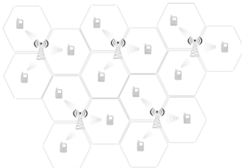
Figure 12. Cellular concept used within mobile telecommunications industry. Each cell corresponds to a geographical region where the radio network of the service provider is able to establish connection with user's devices and provide the service.
