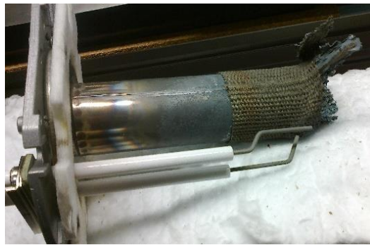
Fig. 3-2: Natural-gas burner head after the accident.
