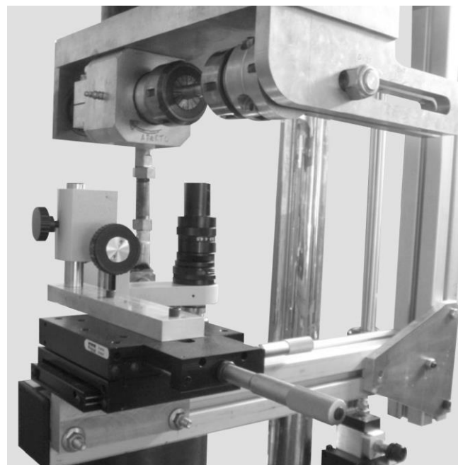
Fig. 2. Fatigue test stand with own-made gripping system
