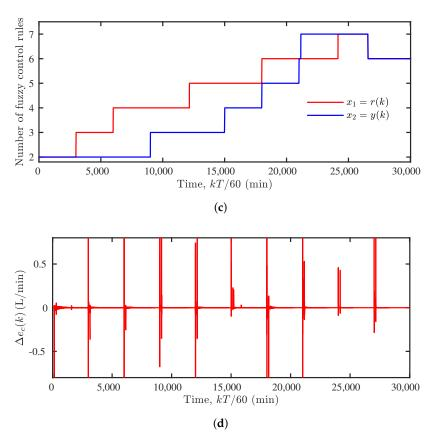
**Figure 4.** Results of the proposed self-evolving FLC design methodology on the CSTR plant. (a) Results of the proposed methodology, and of the SEDFLC method [31]. (b) Command signal of the proposed method and of the SEDFLC method [31]. (c) Evolution of the number of fuzzy control rules. (d) Evolution of  $\Delta e_c(k)$ .
