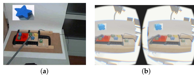
Figure 3. Task 1 setup used to compare performances. The user using a hand stick presses a sequence of key blocks defined by the computer at random. Interface view shows the next block to touch at the upper left corner of the display, after each correct touch. (a) Traditional interface vs. (b) immersive interface.
