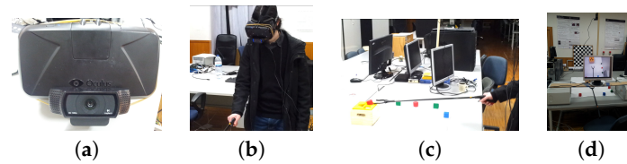
Figure 6. (a) “HMD indirect vision (mono biocular)”: a video see-through HMD; (b,c) user performing a pick and place task using the setup “HMD indirect vision (mono biocular) + gripper”; (d) user performing a pick and place task using the setup “fixed monitor vision (mono biocular) + gripper”.
