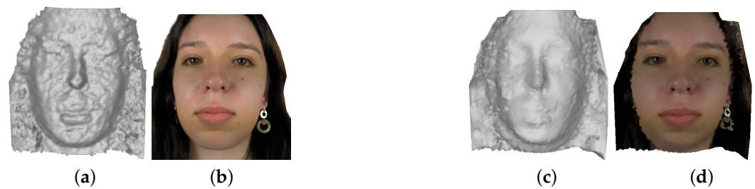
Figure 17. The correction of a mesh obtained using DepthSense camera [43]. We first standardized the scale and sampling frequency in relation to the database, and then we corrected using our filter. Figure (a) shows the acquired noisy mesh, (b) is only the texture, (c) is the filtered mesh and (d) is the filtered mesh with texture.
