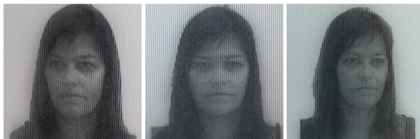
Figure 24. Imprinted lenticular card prototype—these images show the same card viewed from different perspectives.
