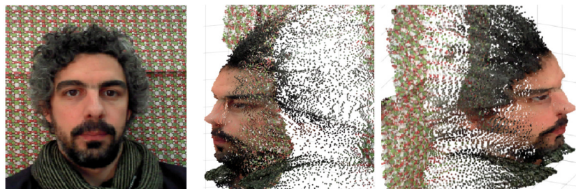
Figure 14. Image and 3D reconstruction views of the point cloud estimated by the DepthSense software.
