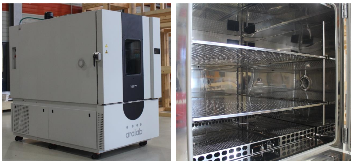
Figure 1. Climatic chamber prototype under development: external and internal view.
