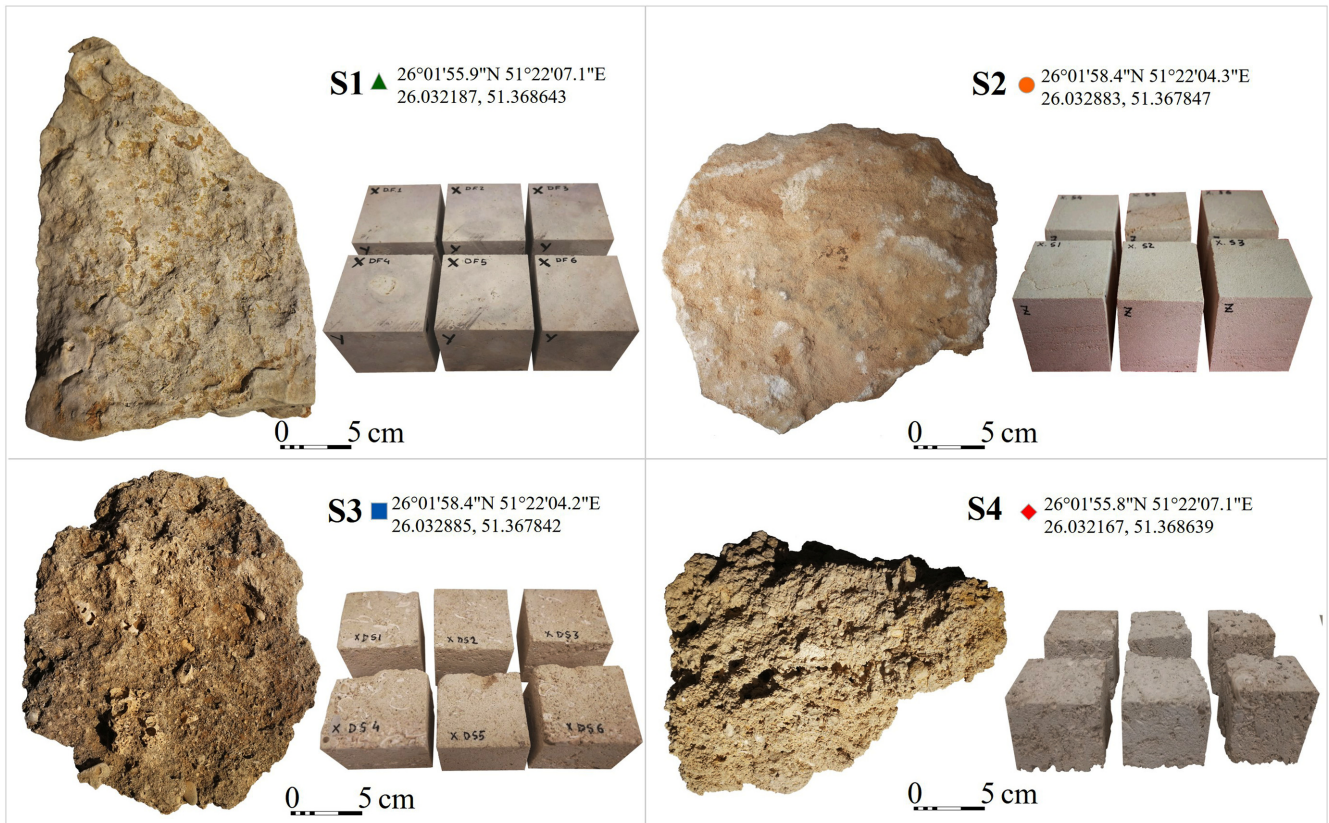
Figure 3. Samples of masonry stones collected at Fuwairit archaeological site and six cubes obtained from each of them for petrophysical analysis.
