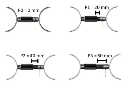
Figure 9. Device positions considered in the tests.
