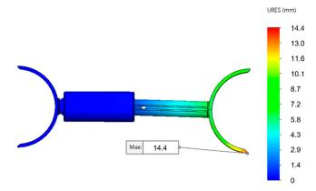
Figure 17. Distribution of resultant displacements for load case 2.
