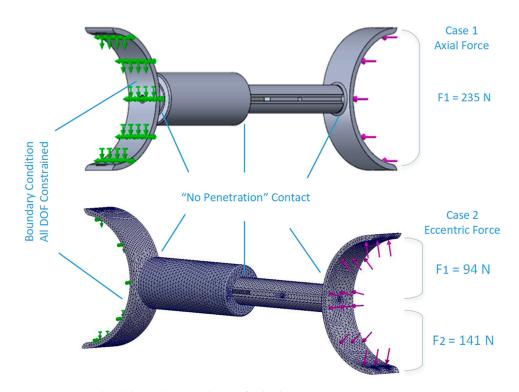
Figure 12. Load and boundary conditions for both situations.
