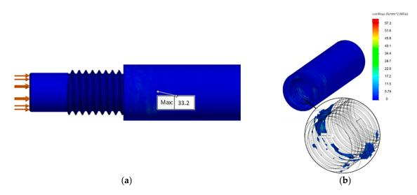
Figure 15. Distribution of von Mises stress for the instrumented device: (a) View of the global model;(b) Detail of von Mises stress distribution in the contact region.
