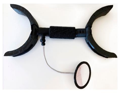
Figure 7. Mechanical device with the mirror system coupled.
