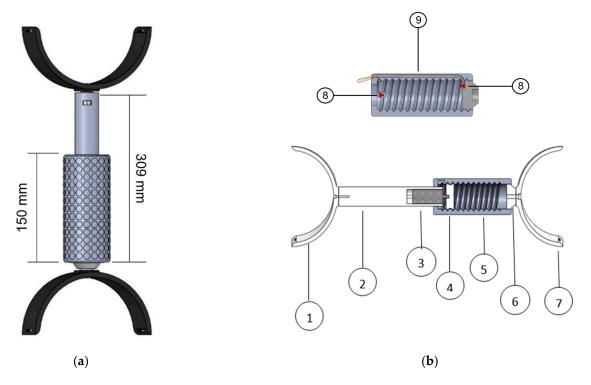
**Figure 4.** 3D model of the motorised device: (**a**) Global visualization; (**b**) Detail with components, (1) motor grip, (2)—movable side element, (3)—DC motor, (4)—threaded element, (5) central element, (6)—fastening element, (7)— fixed grip, (8)—positioning of end limit switches, (9)—embedded wire for signal transport.
