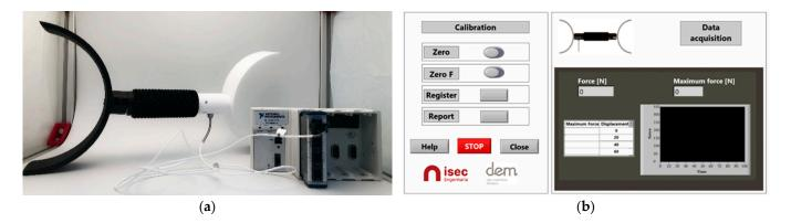
Figure 8. (a) Instrumented device; (b) Interface of Labview program to connect the load cell.
