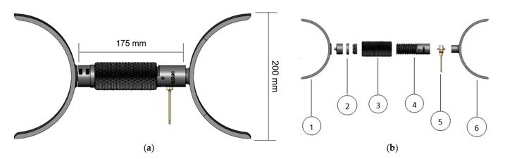
**Figure 3.** 3D model of the instrumented device for force measurement: (**a**) Global visualization; (**b**) Detail with components, (1)—fixed claw, (2)—fixed side element, (3)—central element, (4)—mobile side element, (5)—load cell, (6)—instrumented claw.
