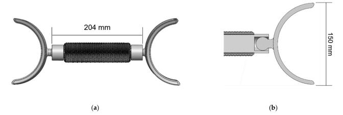
Figure 2. 3D model of the mechanical device: (a) Global visualization; (b) Detail of pivot system.
