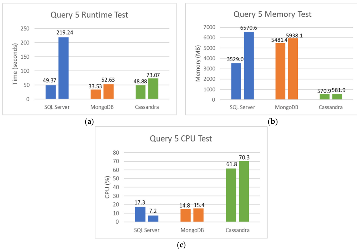
Figure 20. Runtime Test, Memory Test, and CPU Percentage Test for Query 5. (a) Runtime test for Query 5. (b) RAM used for Query 5. (c) CPU Percentage for Query 5.
