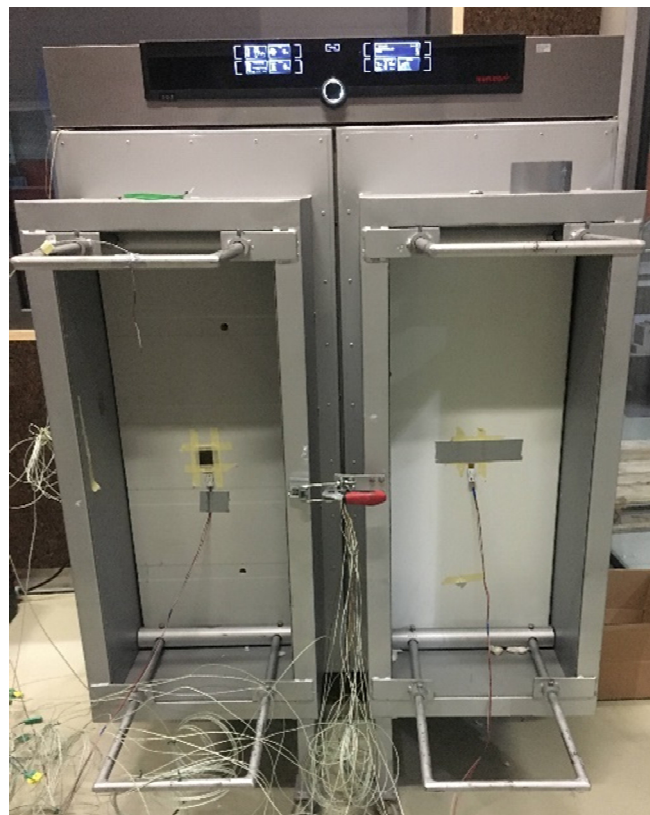
Figure 4. Photographic register of the oven door modifications.
