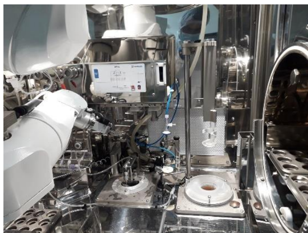
Figure 2.9: Theodorico® robotic arm, performing fractioning and dispensing.
