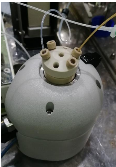
Figure 3.14: PETWave ® microwave cavity with reactor installed.
