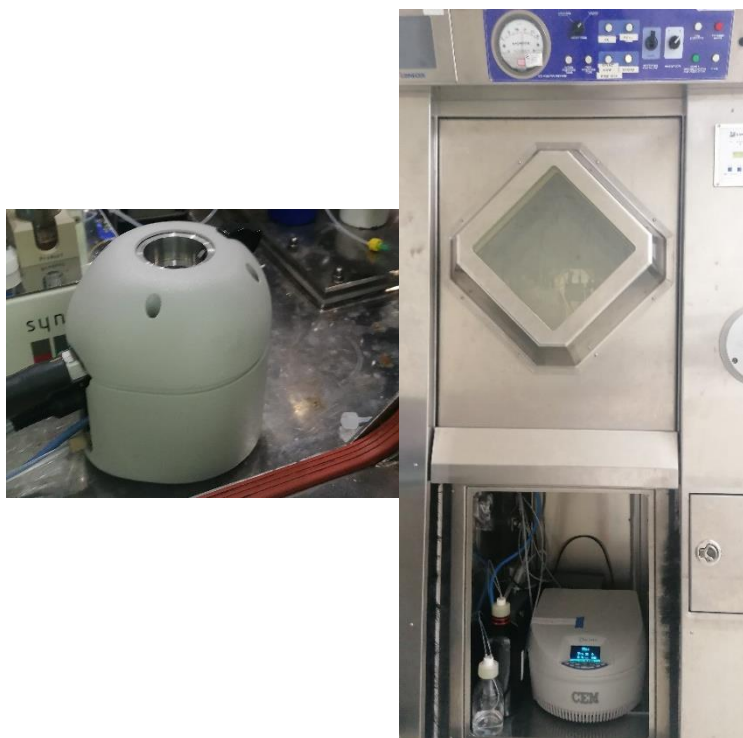
Figure 5.21: MIP1-1P hot cell, microwave system and microwave cavity of PETwave®.
