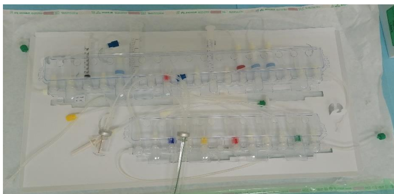
Figure 5.2: Cassette for the production of [ 18 F]FDOPA, supplied by Trasis.
