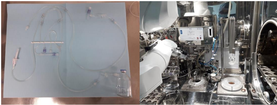
Figure 5.8: Theodorico kit W before installation (left). Theodorico robotic arm after installation of Theodorico kit W (right).
