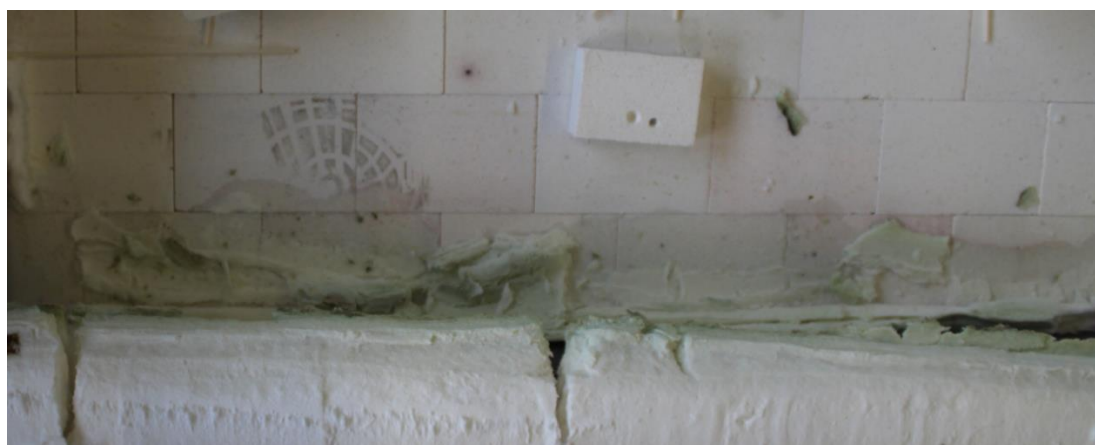
Figure 5-51 – Test series S09.HT.CBJ – Reaction between alumina-spinel bricks and rockwool insulation
