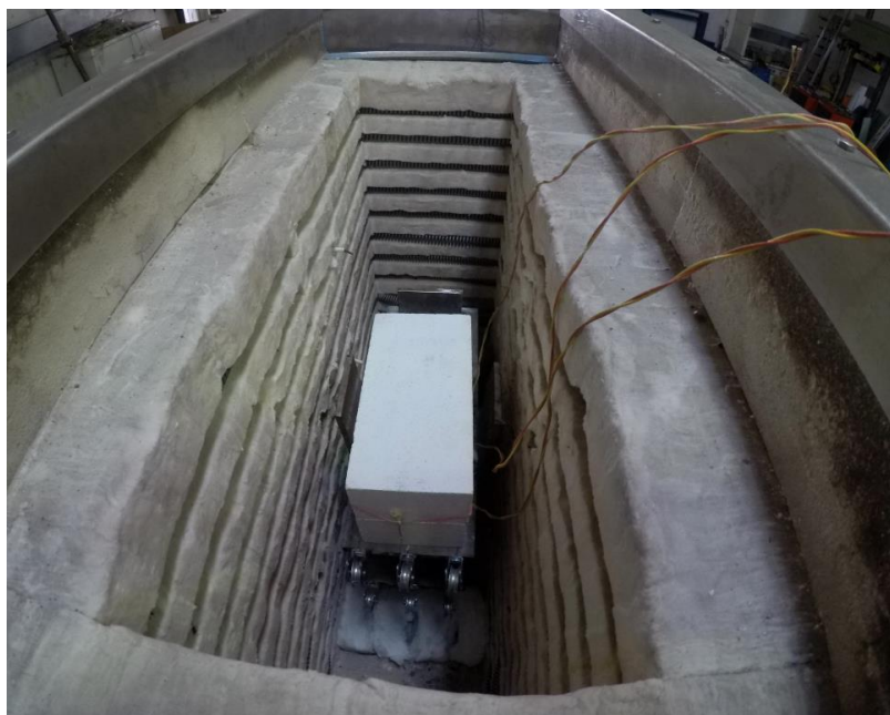
Figure 3-31 – Prism composed by two stacked bricks inside the furnace chamber
