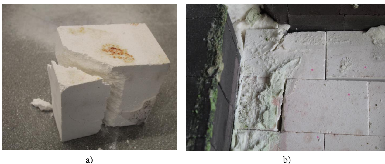
Figure 5-59 – Test series S09.HT.CBJ – Shear failure associated to creep at the brick adjacent to the plunger chamfers
