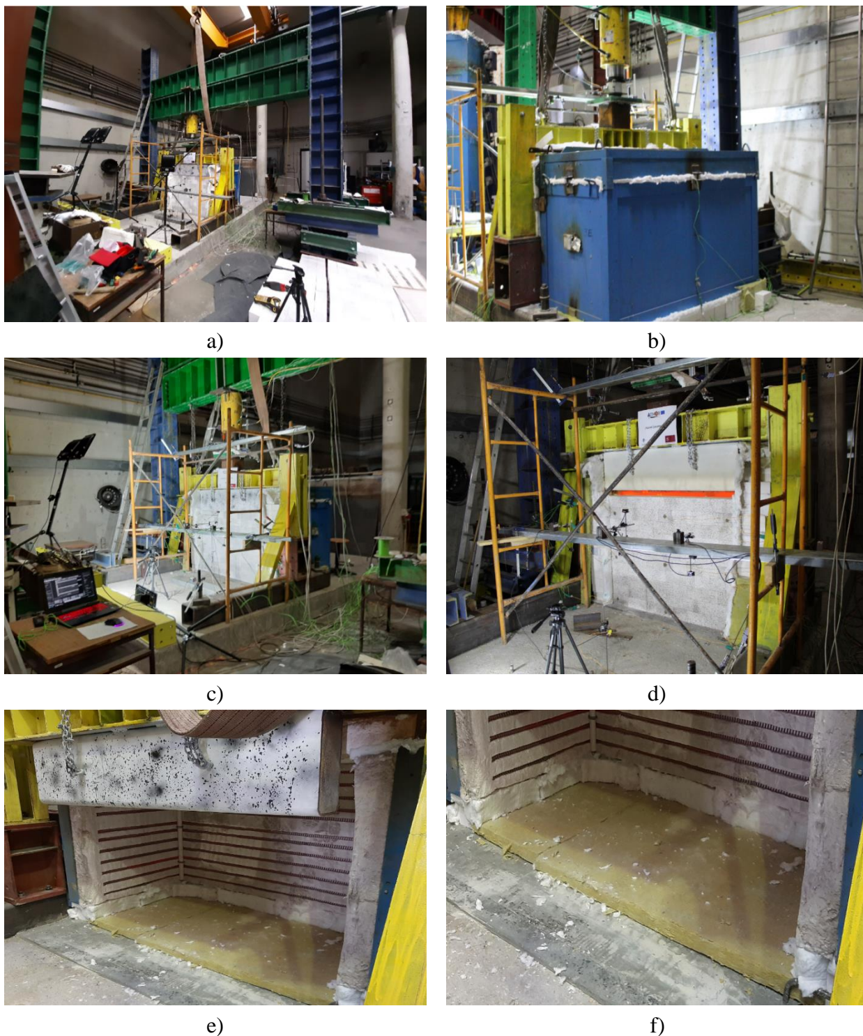
Figure 4-3 – Test set-up at high temperatures: a) General overview of the test setup; b) Back view; c) Specimen in position for testing; d) End of the test; e) Resistances of the furnace; f) Bottom insulation
