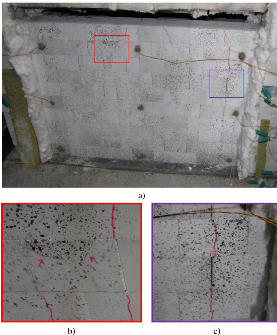
Figure 4-34 – Test series S04.HT.RTE – Overview of vertical cracks in specimen S04.HT.RTE.01; b) Brick crushing due to stress concentrations at the cross joints; c) Brick cracks and joint opening
