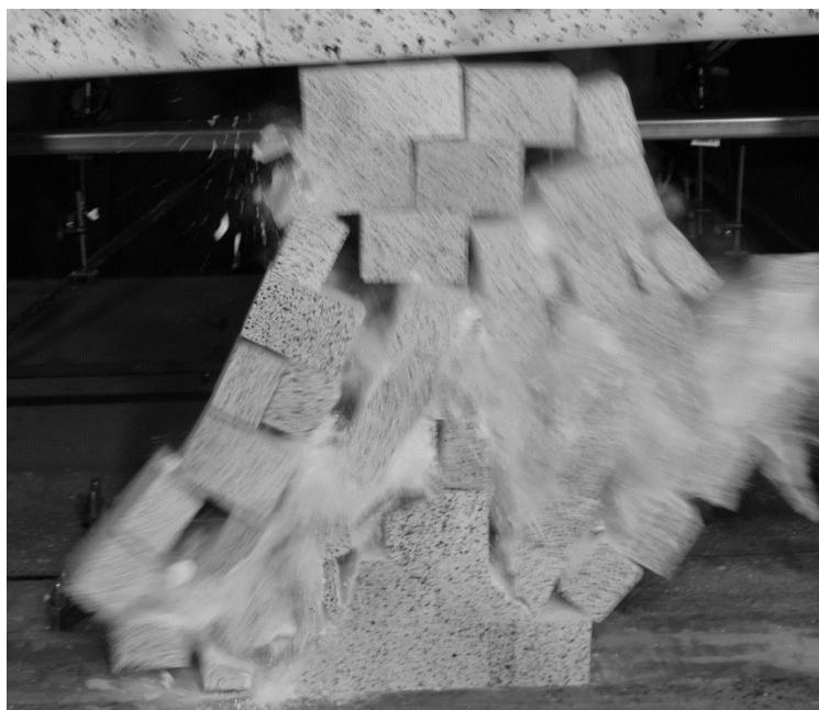
Figure 4-16 – Test series S01.HT.LBC.02 – Specimen failure
