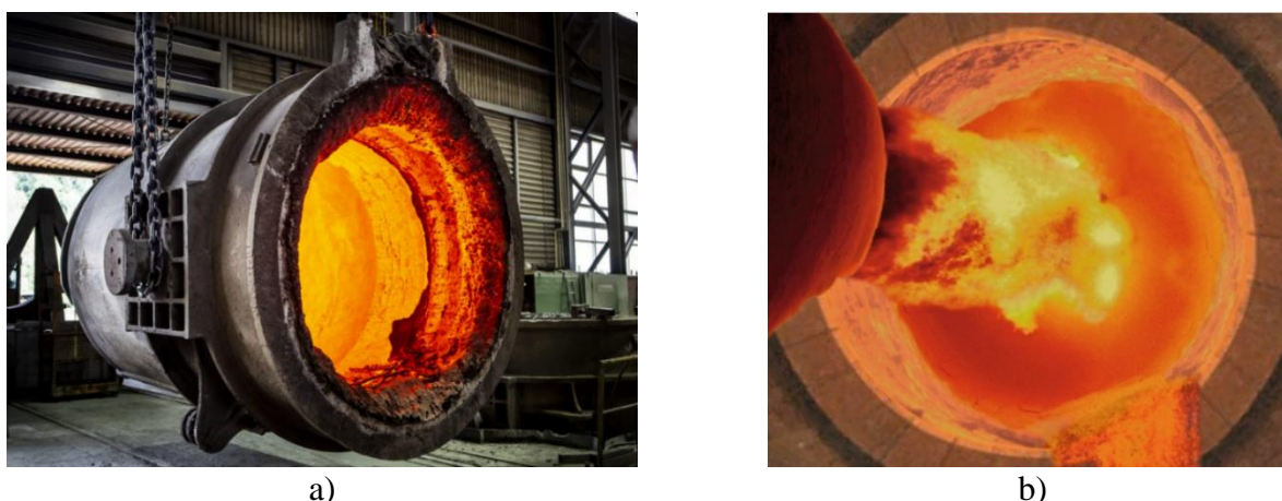
Figure 1-1 – Refractory linings: a) steel ladle (Seven Refractories, 2021); b) rotary cement kiln (ZKG, 2021)
