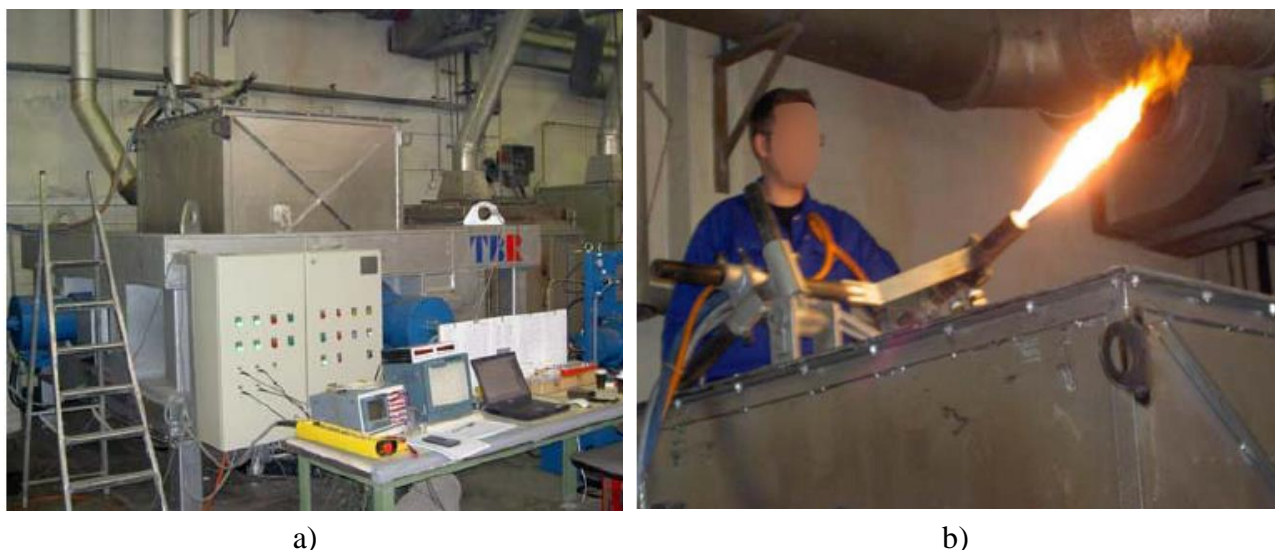
Figure 2-21 – Biaxial press: a) Experimental setup; b) Gas burner (Prietl, 2006)
