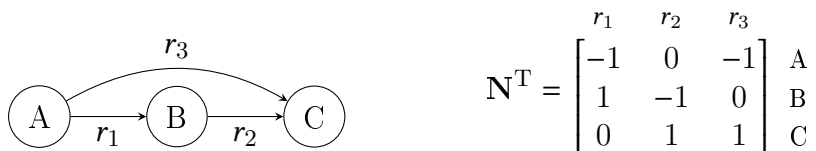
Figure 2.11 Reaction network with a redundant pathway and corresponding stoichiometric matrix.
