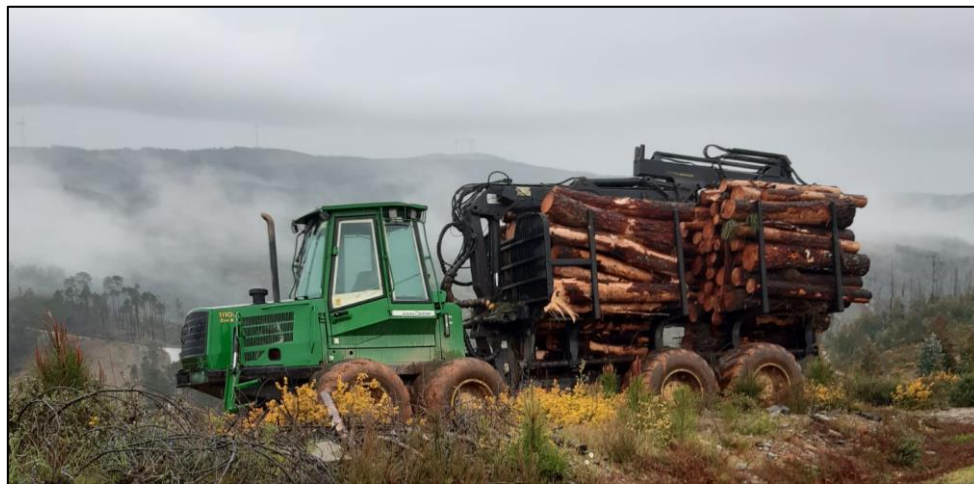
Figure 34 – Forwarding of roundwood with forwarder
