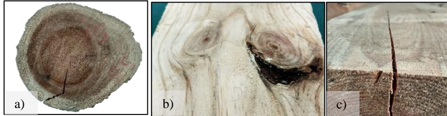
Figure 8 - a) Reaction wood; b) Knots and resin pockets; c) Cracks
