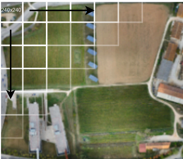
Fig. 5. Orthomosaic splitting approach. The splitting begins at the upper left corner and proceeds to the right until the end of the row. The process is repeated until the bottom.
