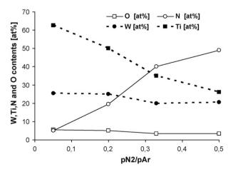
**Fig. 3.** Evolution of the chemical composition of reactively deposited W–Ti–N coatings as a function of the partial pressure ratio of the reactive gas  $(p_{N_2}/p_{Ar})$ .
