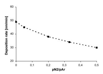
**Fig. 5.** Evolution of the deposition rate as a function of the partial pressure of the reactive gas for IndDep W–Ti–N coatings.
