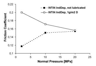
**Fig. 14.** Evolution of the friction coefficient as a function of the applied normal pressure for industrially deposited W–Ti–N coated samples in strip-drawing tests with DDS steel sheets.
