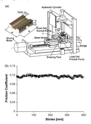
**Fig. 2.** (a) Schematic view of the strip-drawing test equipment. (b) Typical curve of the evolution of the friction coefficient with the stroke during a strip-drawing test – DDS-40G steel sliding against an uncoated D2 steel tool with  $2\,g\,m^{-2}$  of lubricant A under 5 MPa normal pressure.
