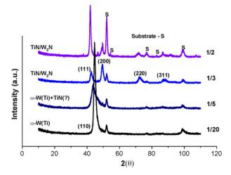
**Fig. 6.** XRD patterns of IndDep W–Ti–N coatings deposited with increasing partial pressure of the reactive gas ( $p_{N_2}/p_{Ar} = 1/20, 1/5, 1/3, 1/2$ ).
