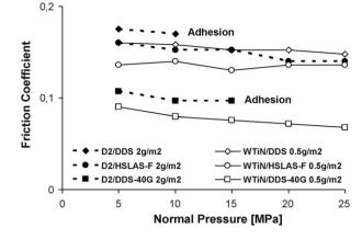
**Fig. 11.** Friction coefficient in lubricated contact (lubricant D) of uncoated and W–Ti–N coated D2 steel sliding against different sheet materials.
