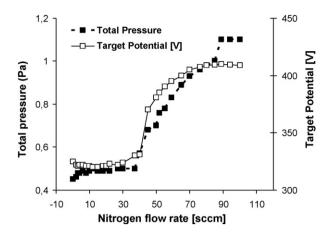
**Fig. 4.** Evolution of the target potential  $(V_t)$  and discharge pressure  $(p_{dep})$  with increasing nitrogen flow rate in an experiment carried out in a reactive discharge with the puzzle W + Ti target. The sudden increases of  $V_t$  and  $p_{dep}$  are typical of target poisoning during Ti deposition.
