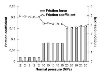
**Fig. 13.** Friction forces and coefficients obtained for industrially deposited W–Ti–N coated samples in strip-drawing tests performed in lubricated conditions (lubricant D) with DDS steel sheets.
