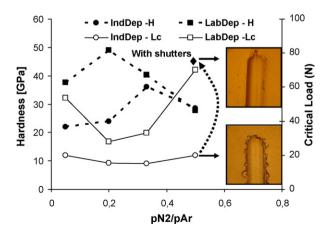
**Fig. 7.** Hardness (H) and scratch-test critical loads (Lc) of W–Ti–N coatings as a function of the N content. The experimental point marked with the ♦ symbol is related to a coating deposited with shutters in front of the targets. The micrographs correspond to the end of the scratch tracks.
