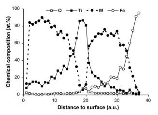
Fig. 8. Depth profiling chemical composition analysis of a W–Ti very thin film evaluated by Auger spectroscopy.
