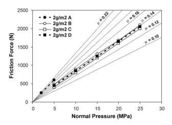
**Fig. 9.** Evolution of the friction force as a function of the normal applied pressure for a DDS steel sliding against an uncoated D2 steel tool.
