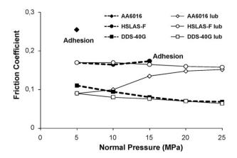
**Fig. 12.** Friction coefficient of different sheet materials sliding against D2 steel coated with a W–Ti–N film in dry and lubricated (lubricant D) conditions.
