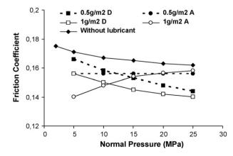
**Fig. 10.** Evolution of the friction coefficient as a function of the normal applied pressure for the DDS steel sliding against a W–Ti–N coated D2 steel tool.
