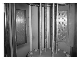
**Fig. 1.** Inside of the deposition chamber of the semi-industrial PVD equipment showing the puzzled target with round pieces of W (25 mm diameter) embedded in the Ti target ( $325 \text{ mm} \times 750 \text{ mm}$ ).
