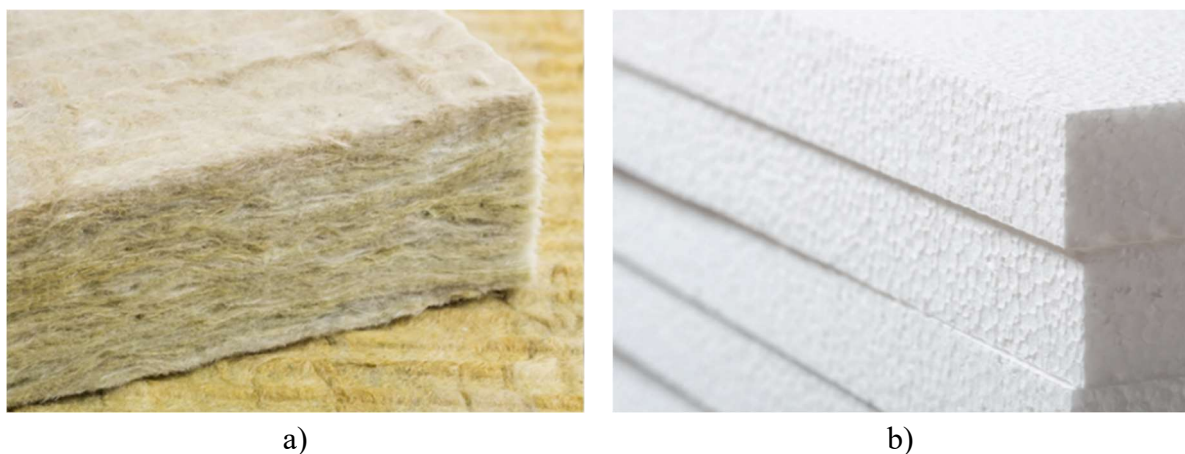
Figure 7 – Thermal insulation materials: a) mineral wool (Termolan, 2021); b) expanded polystyrene (Thermal-engineering, 2021).
