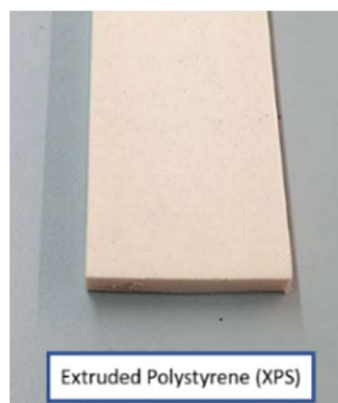
Figure 42 – Extruded polystyrene (XPS) thermal break strip.
